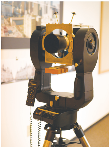
Figure 2: The Meade LX200 adapted to shoot Gigapixel images.
